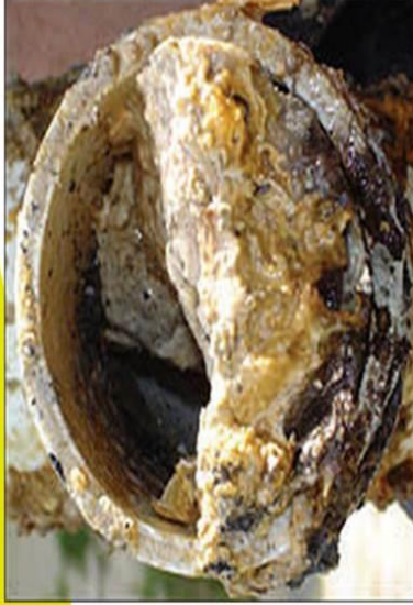
FOG build-up in sewer pipes (shown below) is costly to clean requiring local Public Works staff to go to the site & remove
