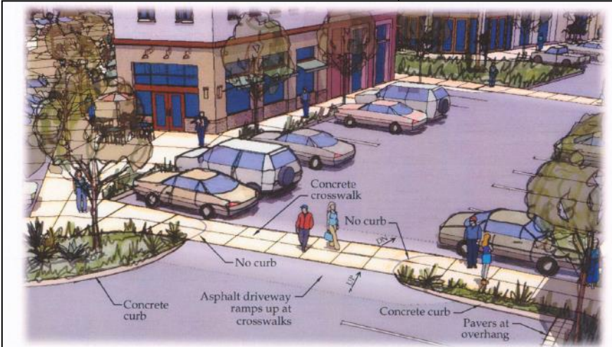
Sketch of Typical Raised Crosswalk Crosswalks throughout project are raised as shown to improve pedestrian safety and convenience.
