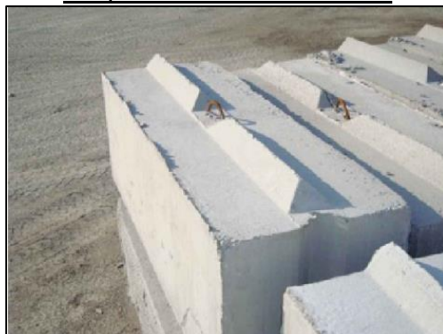
Proposed concrete barrier
