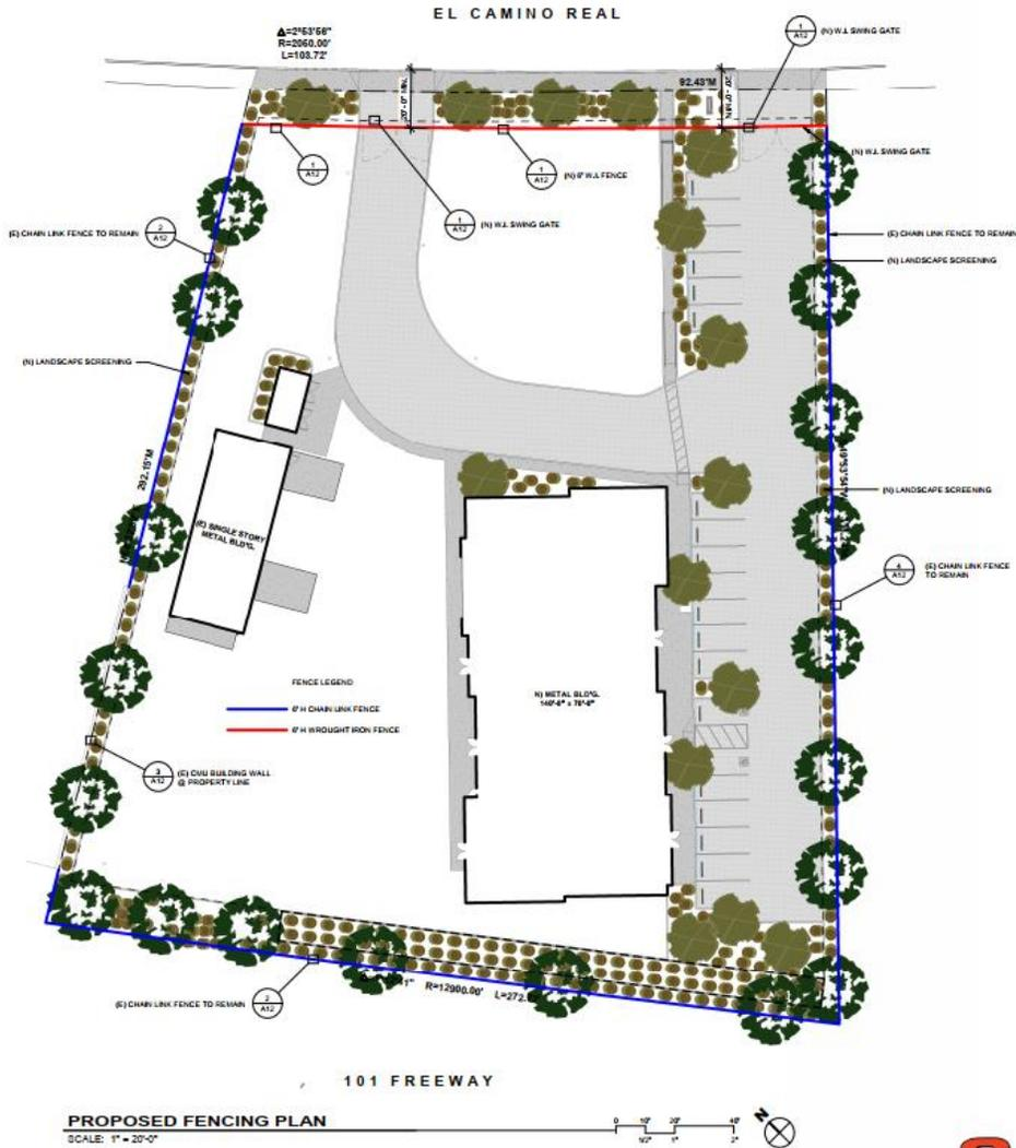
EXISTING 6' HIGH CHAIN LINK FENCE WITH EXISTING GREEN SLATS TO REMAIN. EXISTING RAZOR WIRE ABOVE FENCE IS NOT ALLOWED PER MUNICIPAL CODE STANDARDS. THE RAZOR WIRE NEEDS TO BE REMOVED PRIOR TO FINAL OCCUPANCY.
