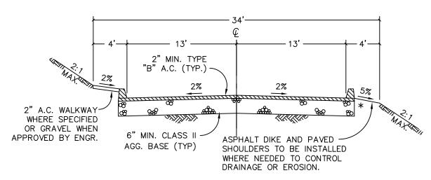
\* NOTE: AS AN ALTERNATE THE CHOKER CAN BE ELIMINATED AND THE AGG. BASE CARRIED TO THE HINGE POINT.
