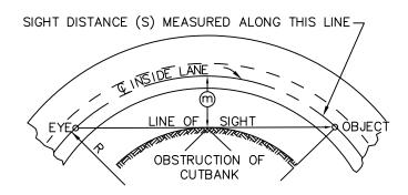
HEIGHT OF EYE = 3.50 ....HEIGHT OF OBJECT = 0.50 FEET LINE OF SIGHT IS 2.0 FEET ABOVE  $\mathbb Q$  INSIDE LANE AT POINT OF OBSTRUCTION
